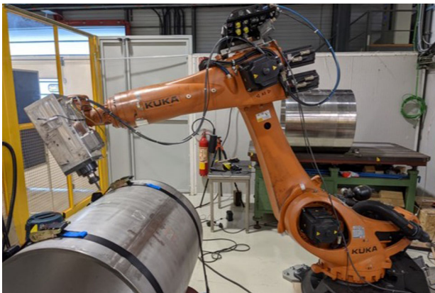
FIG. 15. KUKA KR 120 R2700 HA robotic arm performing a milling test on one of the vessel mockups.
