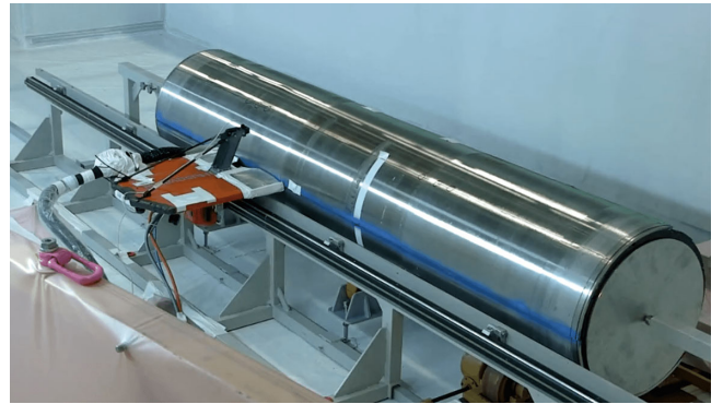
FIG. 22. Longitudinal cutting setup with tailstocks and aluminum discs installed to stabilize the LD sector during cutting, along with the longitudinal guide frame and saw.
