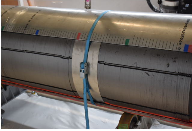
FIG. 23. View of the LD sector resting on the duplex stainless-steel shell after two longitudinal cuts, prior to its replacement with an aluminum shell. The aluminum shell is marked with tape to indicate the extraction positions for the expanded graphite sheets for further postirradiation examination.
