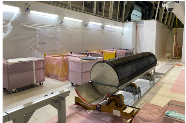
FIG. 25. View of the working conditions implemented during the sheet extraction. The LD sector is supported by the Al sleeve, with Al discs placed on either side to keep the sheets from tipping over. A fastening device attached to the aluminum sleeve was used to secure the discs. Behind the LD sector is a table used for dose measurements, with waste-disposal containers visible in the background.
