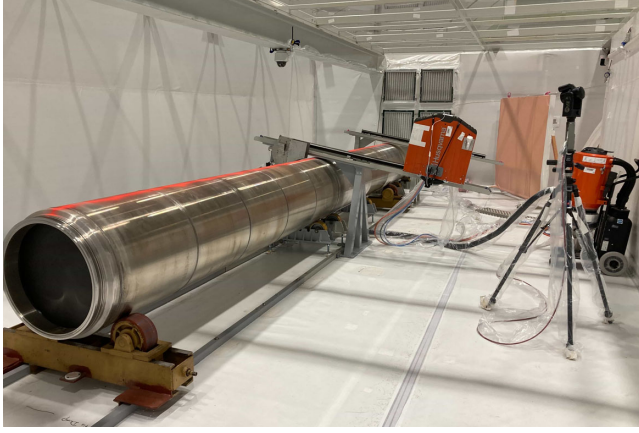
FIG. 19. View of the cutting setup inside the bunker prior to the first two circumferential cuts. The guiding rails are installed in their correct axial positions on either side of the LD sector.
