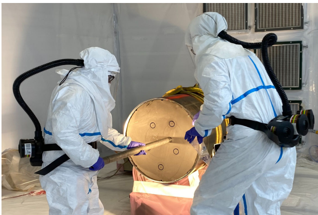
FIG. 32. Extraction process of specimens from the HD blocks. A dedicated pipe was used to break off the corings.
