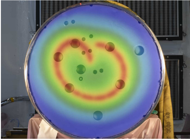
FIG. 30. View of the downstream face of the upstream HD block after specimen extraction, overlaid with corresponding beam sweep to indicate corings from different energy densities.
