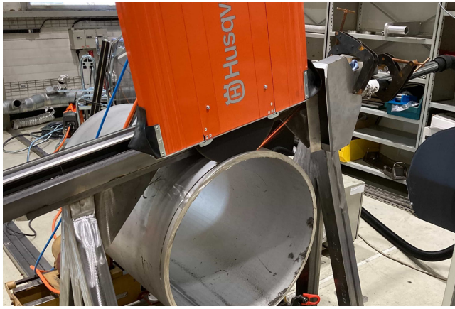
FIG. 16. Husqvarna WS 220 saw [39] installed on the inclined guiding frame while performing a circumferential cutting trial on one of the vessel mockups.
